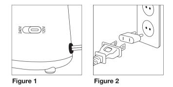
**NOTE:** Use the proper adaptor plug to make the connection to a 220/240 volt electrical outlet (Figure 2).
