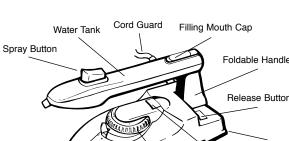
Temperature Indicator Light Steam "ON-OFF" Sole Plate Control Knob Switch
